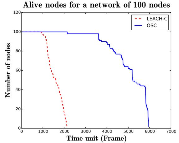
Figure 2. Alive nodes for a homogeneous network of 100 nodes.
