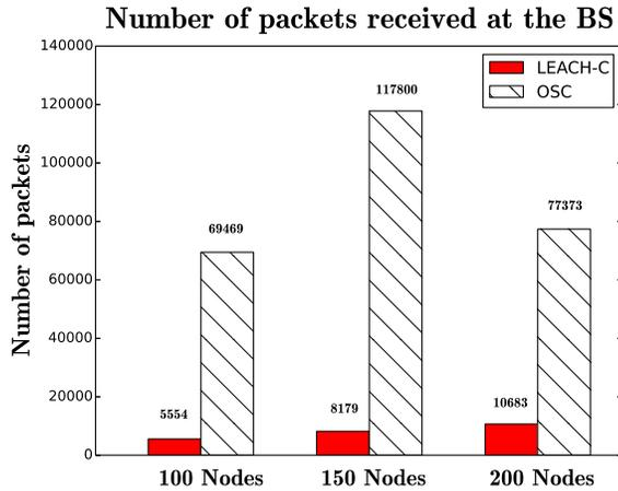
Figure 5. Packet received for homogeneous networks.
