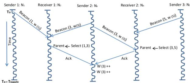
Fig. 2. *The Least Interference Beaconing Protocol*
