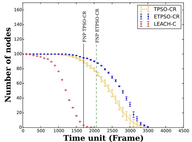
Figure 14. Alive nodes for heterogeneous networks of 100 nodes.
