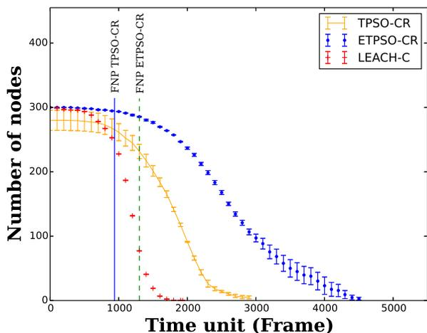
Figure 16. Alive nodes for heterogeneous networks of 300 nodes.
