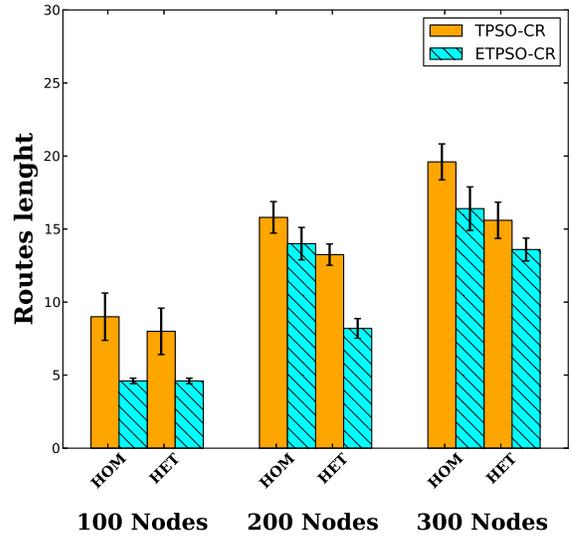
Figure 4. Example of the mean of routes' lengths in one round for homogeneous (HOM) and heterogeneous (HET) networks.
