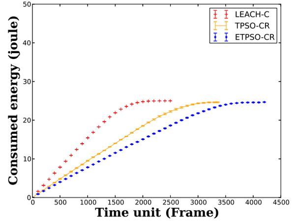
Figure 10. Energy consumption vs. time for homogeneous networks of 100 nodes.
