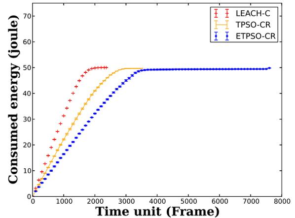
Figure 11. Energy consumption vs. time for homogeneous networks of 200 nodes.
