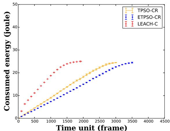
Figure 18. Energy consumption vs. time for heterogeneous networks of 100 nodes.
