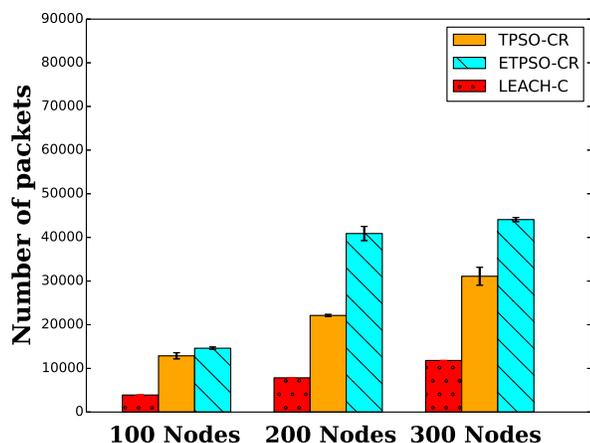
Figure 17. Total number of received data at the base station in heterogeneous networks.
