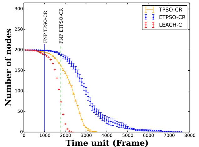
Figure 7. Alive nodes vs. time for homogeneous networks of 200 nodes.
