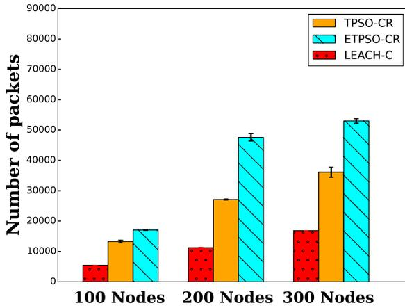
Figure 9. Total number of received data at the base station in homogeneous networks.
