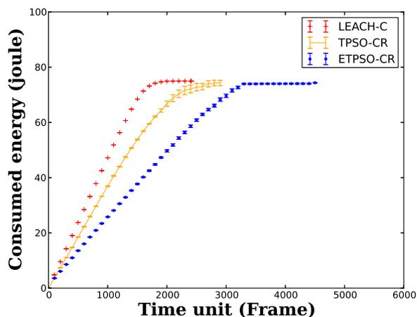
Figure 19. Energy consumption vs. time for heterogeneous networks of 100 nodes.
