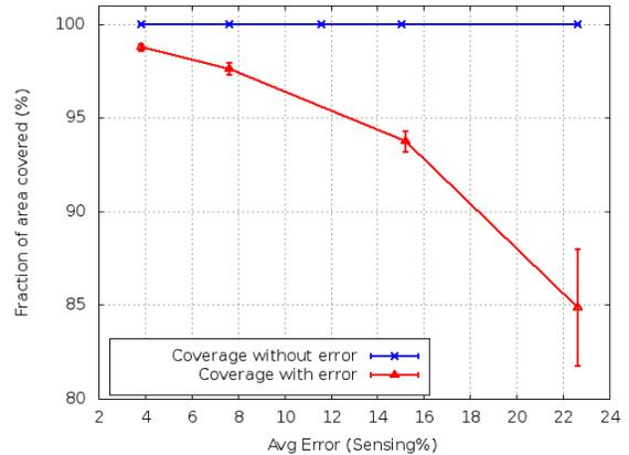
Fig. 1. Quantifying the effect of localization errors on coverage
