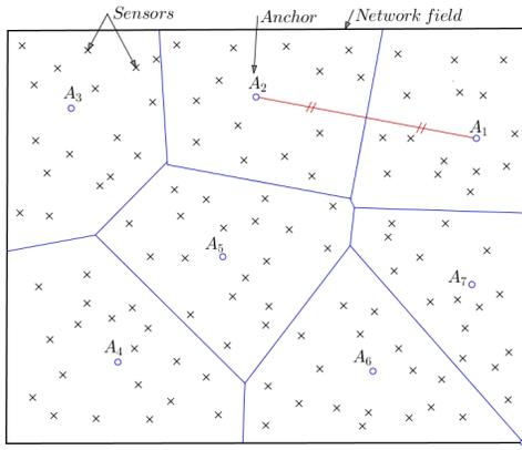
Fig. 5. Network field subdivided into 7 Cells using Voronoi Diagram. The formation of the Voronoi diagram is done through the coordination among the anchors
