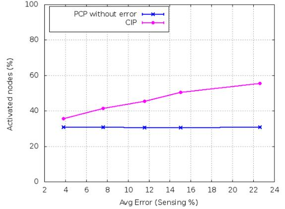
Fig. 9. The effect of average localization error on the fraction of activated nodes required for achieving full area coverage
