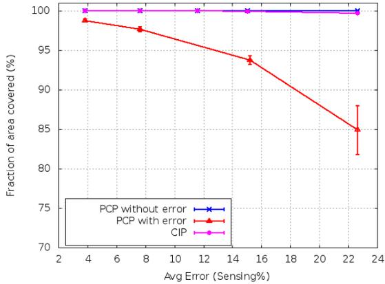
Fig. 8. The effect of localization error on coverage under CIP and the baseline approaches
