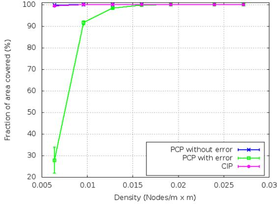
Fig. 7. The fraction of area covered while varying the node density
