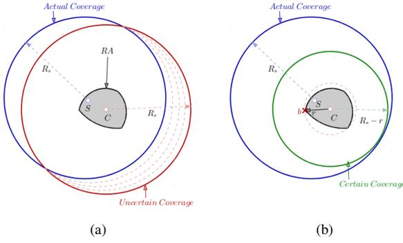
Fig. 3. Sensors coverage estimation: (a) Uncertain coverage without adjustable sensing range. (b) Certain coverage range using an adjusted sensing range
