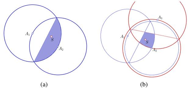
Fig. 2. Illustrating the residence area in HSL using: (a) two anchors, and (b) three anchors
