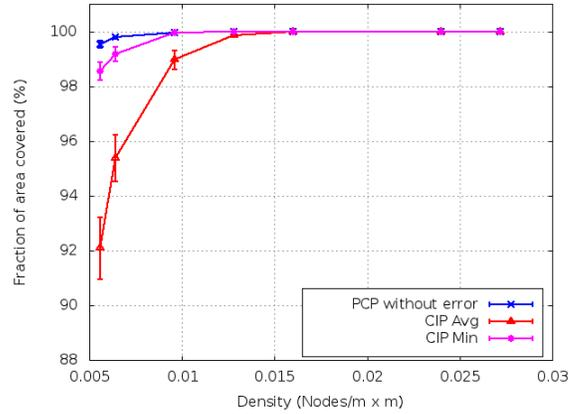
Fig. 10. Comparing the effect of using minimum and average errors on coverage as the node density changes
