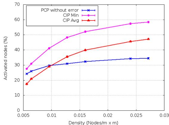
Fig. 11. The percentage of activated nodes for the various node densities when average and minimum errors are factored
