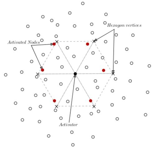
Fig. 6. The activation process based on triangular lattice
